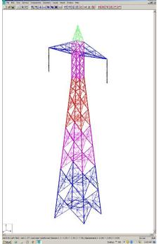
Design of 500kV HVDC Semnan – Golpayegan Lattice Tower by PLS-TOWER
